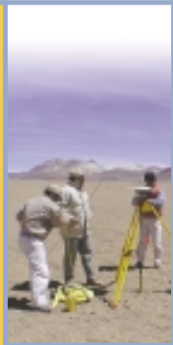
Using the Global Positioning System to mark a location at the ALMA site.
